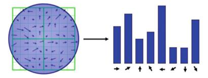
Fig. 5 Histogram of oriented gradients
