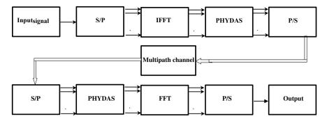
Fig. 5 FBMC block diagram
