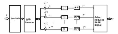
Fig. 9 Proposed SLM technique
