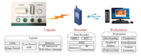
Fig. 2 Capsule endoscopy system [7]
