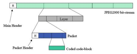
Fig. 14 JPEG 2000 bitstream and the structure of the layer
