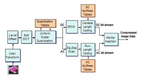
Fig. 6 JPEG algorithm encoding
