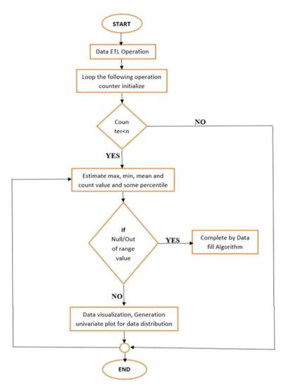
Fig. 5 The flowchart of algorithm applied
