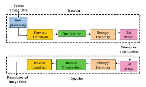
Fig. 12 JPEG 2000 compression engine
