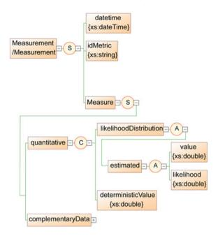
Fig. 4 The measurement tag in the CINCAMI/MIS message
