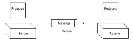
Fig. 5 Components of data communication
