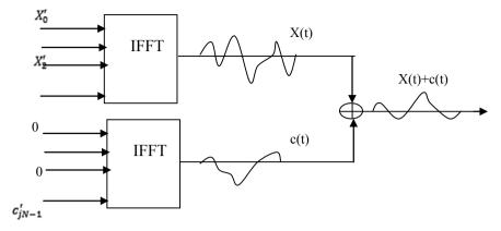
Fig. 7 Block diagram for TR
