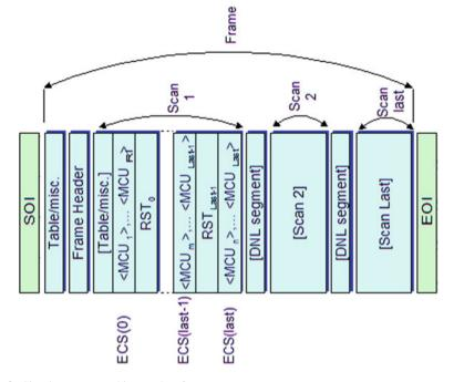
Fig. 9 Simple compressed image data format
