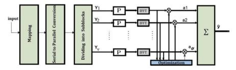
Fig. 8 Proposed modified PTS technique
