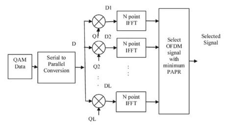
Fig. 6 Selected mapping OFDM system
