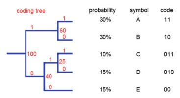
Fig. 2 Huffman encoding procedure
