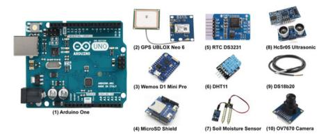
Fig. 14 Set of components based on the Arduino one used for building the monitoring station
