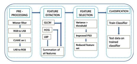
Fig. 4 Brief idea of the system for automatic detection of ulcer
