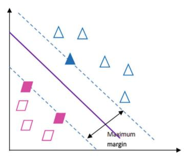
Fig. 5 Support vector machine classification
