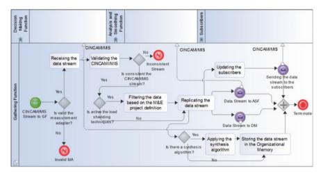
Fig. 10 The data gathering process using BPMN notation
